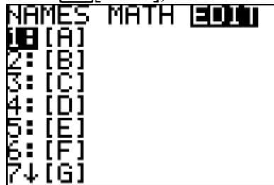
Enter the size of the matrix: **2x3** for our example (2 rows by 3 columns). Then enter your values in the augmented matrix. Press **[ENTER]** after each value or use the arrow keys to go from one position to the next in the matrix.
