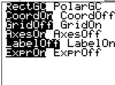
The calculator will primarily remain in these settings for the format menu. **RectGC** displays the cursor location as rectangular coordinates X and Y. **CoordOn** displays the cursor coordinates at the bottom of the graph. **GridOff** does not display grid points. **AxesOn** displays the axes. **LabelOff** does not display labels (X and Y) for the axes. **ExprOn** will display the Y= expression when the trace cursor is active.
