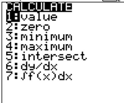
**Value** evaluates a function for a specified value of X. **Zero** finds the x-intercept of a function. **Minimum** finds the minimum value of a function within a specified interval. **Maximum** finds the maximum value of a function within a specified interval. **Intersect** finds the coordinates of a point at which two or more functions intersect.
