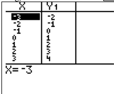
The table feature shows the coordinates of the function that has been entered for  $Y_1$ . ( $Y_1 = X + 1$  in this example.)
