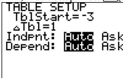
Along with the table feature in part g) above, the initial value for the independent variable can be specified using **TblStart** and  $\Delta Tbl$  defines the increment for the independent variable. When **Indpnt** and **Depend** are set to **Auto**, the values are displayed automatically in both the independent-variable column and in all dependent-variable columns.
