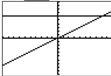
To find the solution, press  $\boxed{2nd}$  $\boxed{[CALC]}$  and select #5 **Intersect**. Since we only have two functions graphed, the calculator will go to  $Y_1$  as the first curve (press  $\boxed{ENTER}$ ),  $Y_2$  as the second curve (press  $\boxed{ENTER}$ ), and arrow close to the intersection point for a guess (press  $\boxed{ENTER}$ ). See the illustration below:
